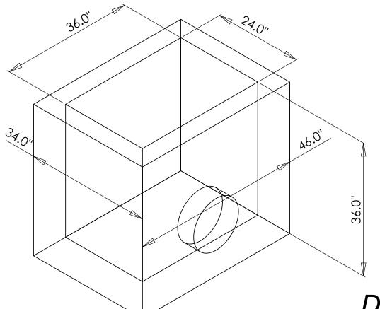
Standard 2' x 3' x 3' curb inlet box. This particular drawing fits a 14" opening in a typical location. Other holes can be poured in.
